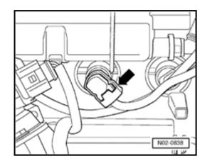
If spark plug connector is equipped with tool for removal of spark plug connectors -arrow-, remove it.
