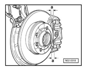
a - Pad thickness including backing plate
