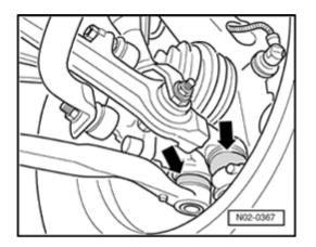
Control arm joints, checking
