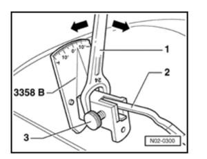
If necessary adjust contact angle to specified value as follows:
