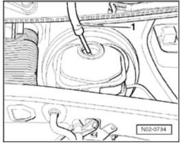
Using suction hose -1- from VAS 5234 remove as much brake fluid from the reservoir as possible.
