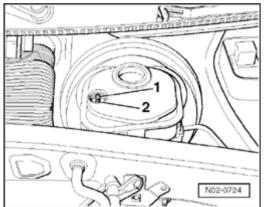
Remove cap -arrow- of brake fluid reservoir by turning.
