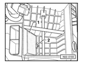
Depending on the model, a screen -1- is installed in lower part close to the air intake channel.
