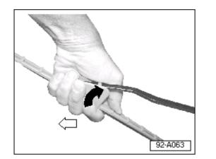
Rotate blade in opposite direction (black arrow) then, carefully slide blade off wiper arm.
