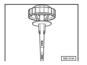
If fluid level is above the mark, some fluid must be siphoned off.
