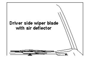
Wiper blade with air deflector (arrow) must be installed on driver's side with deflector on bottom of wiper blade.
