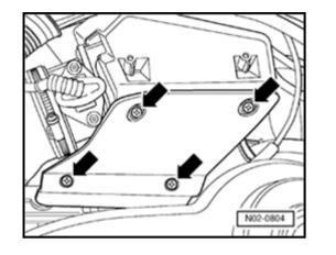
If applicable, install heat shield and secure with screws -arrows-.
