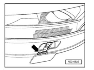
Pull spray jets out to stop and adjust spray to the applicable points using adjustment tool 3019 A.
