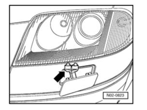
Pull spray jets out to stop and adjust spray to applicable points using adjustment tool 3019 A.
